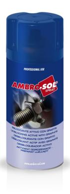
HOW TO USE Shake well before use. Spray the product on the part to be treated, leave for a few minutes, then in the case of rusted parts proceed to unlock, with resistant incrustations repeat. The product can also be sprayed with drinking straw Modular (inserted in the cap multi-straw). PRECAUTIONS: Do not apply to equipment in tension. Do not apply to materials overheated.
