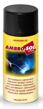
HOW TO USE Before applying thoroughly clean the torch from existing slag and subsequently apply the product. Spray onto the mouth of the torch and the edges of the surface to be welded. Do not spray directly on the edges to be welded. Shake the bottle before use. Making your first vacuum splash if the can is new. Keep the cylinder 20-30 cm away from the surface and in vertical position. Do not spray an excessive amount of product.
